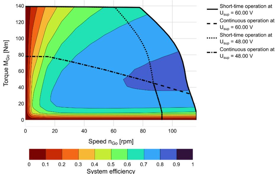
Note: This graphic shows the maximum achievable joint torque/velocities for the given supply voltages. Refer to the *Power Conversion Characteristics* table above for details about the continuous operating points. Further details are available on request.
